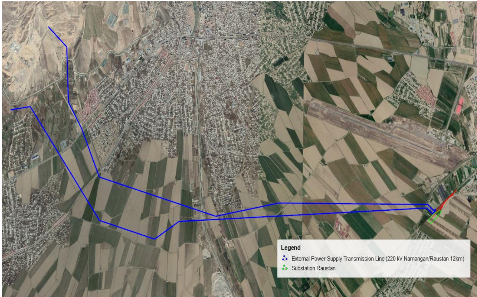
Figure 1.3: Schemes of External Power Supply Transmission Line (220 kV Namangan/Raustan 12km)
